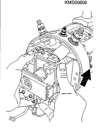
Completely disassemble connections term. 30, term. 31 and term. 48 (1). NOTE: For term. 30 and term. 31, only unfasten nut inside commutator end shield (arrows).
